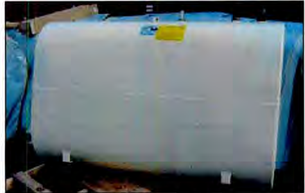
5.2 Epoxy-coated 1,135 litre (250 gallon) heating oil tank.
