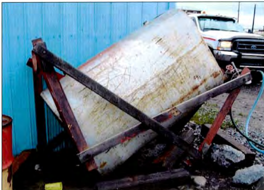
4.4b This heating oil tank was resting on a wood-metal stand, which eventually collapsed under the weight of the tank, spilling 445 litres (100 gallons) of heating oil onto the ground.
