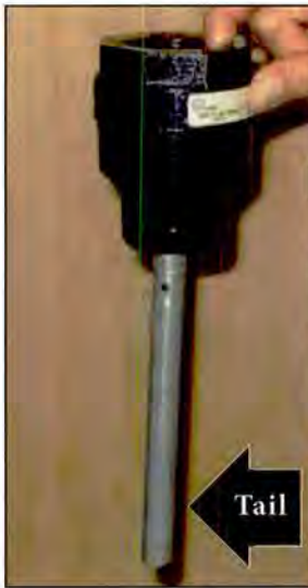
4.8a Heating oil tank vent whistle: the tail of the vent whistle protrudes into the oil tank; the vent pipe screws into the top of the vent whistle.
